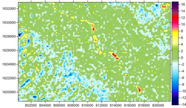
**Fig. 4.** The distribution map of PALSAR backscatter coefficient subtraction value ( $\Delta\sigma_t^0$ ) between September 15<sup>th</sup>, 2009 and September 10<sup>th</sup>, 2007 of Kassala area (where, the changes of surface roughness (mesquite tress pixels) ranged the values of ( $0 \leq \Delta\sigma_t^0 \leq +4$ ) and the changes of soil moisture (bare soil or river channel pixels)) are ( $+4 < \Delta\sigma_t^0$ ) or ( $0 > \Delta\sigma_t^0$ )).
