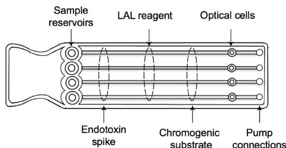
Fig. 1. The Endosafe<sup>®</sup> PTS<sup>™</sup>. The limulus amoebocyte lysate (LAL) spectrophotometer (upper) and reagent cartridge (bottom) for PTS<sup>™</sup>.
