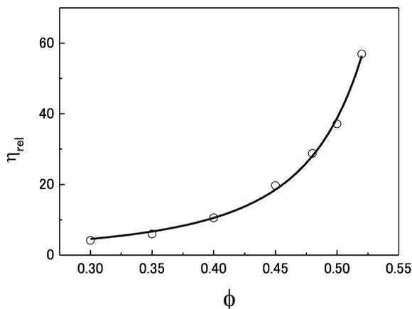
**Fig. 7** Volume fraction dependence of relative viscosity for the model chocolate containing lecithin (0.5 wt%) at a high shear rate ( $125 \text{ s}^{-1}$ ). The line denotes the prediction of the Krieger-Dougherty equation (Eq. 3).
