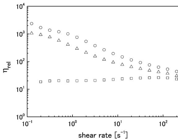
**Fig. 5** Flow curves of the model chocolate ( $\phi=0.5$ ). Circles denote the results of the control (no emulsifier), triangles and squares denote the results of samples containing lecithin and PGPR, respectively. The concentrations of lecithin and PGPR were 0.5 wt%.
