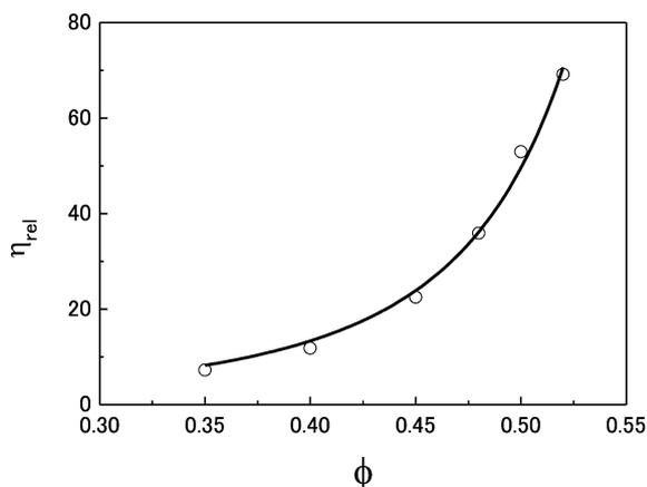
**Fig. 3** Volume fraction dependence of relative viscosity of the model chocolate without emulsifier at a high shear rate ( $125 \text{ s}^{-1}$ ). The line denotes the prediction based on the Krieger-Dougherty equation (Eq. 3)
