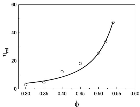
**Fig. 8** Volume fraction dependence of relative viscosity for the model chocolate containing PGPR (0.5 wt%) at a high shear rate ( $125 \text{ s}^{-1}$ ). The line denotes the prediction of the Krieger-Dougherty equation (Eq. 3)
