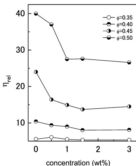
**Fig. 9** The relative viscosity for the model chocolate with various volume fractions of silica particles containing ER-290.  $\phi$  denotes the volume fraction of silica particles in the system. The viscosities were measured at  $125 \text{ s}^{-1}$  and  $50 \text{ }^\circ\text{C}$ .
