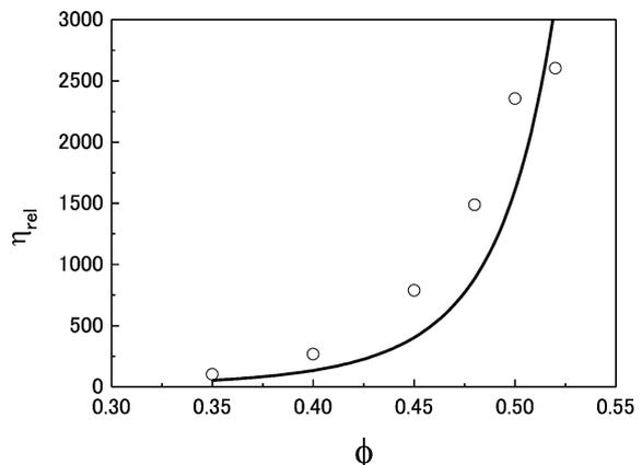
**Fig. 4** Volume fraction dependence of relative viscosity for the model chocolate without emulsifier at a low shear rate ( $1.25 \text{ s}^{-1}$ ). The line denotes the prediction based on the Krieger-Dougherty equation (Eq. 3)
