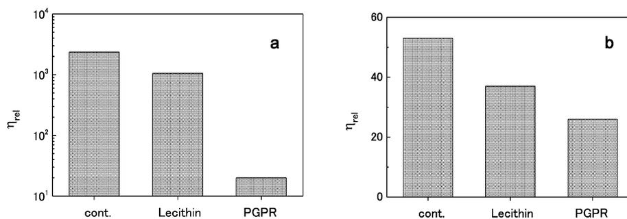
**Fig. 6** Effect of emulsifiers on relative viscosity at  $0.125 \text{ s}^{-1}$  (a) and  $125 \text{ s}^{-1}$  (b) for the model chocolate. The concentration of both lecithin and PGPR was 0.5 wt%.
