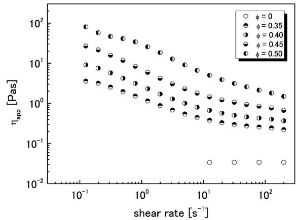
Fig. 2 Flow curves of the model chocolate with various volume fractions of silica particles at 50 °C.  $\phi$  denotes the volume fraction of silica particles in the system, where  $\phi = 0$  denotes molten cocoa butter.
