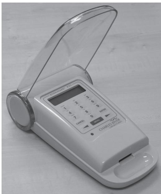
Fig. 1. The Endosafe<sup>®</sup> PTS system. Spectrophotometer and reader.
