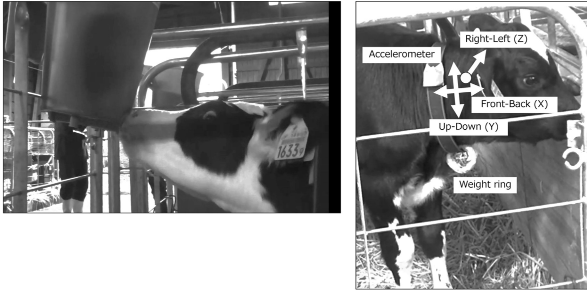
Fig.1. (Left) Milk replacer was fed from a bucket with a rubber teat. The bucket was suspended on a fence. (Right) The three-dimensional accelerometer was attached at right side on the collar with a weight-ring.
