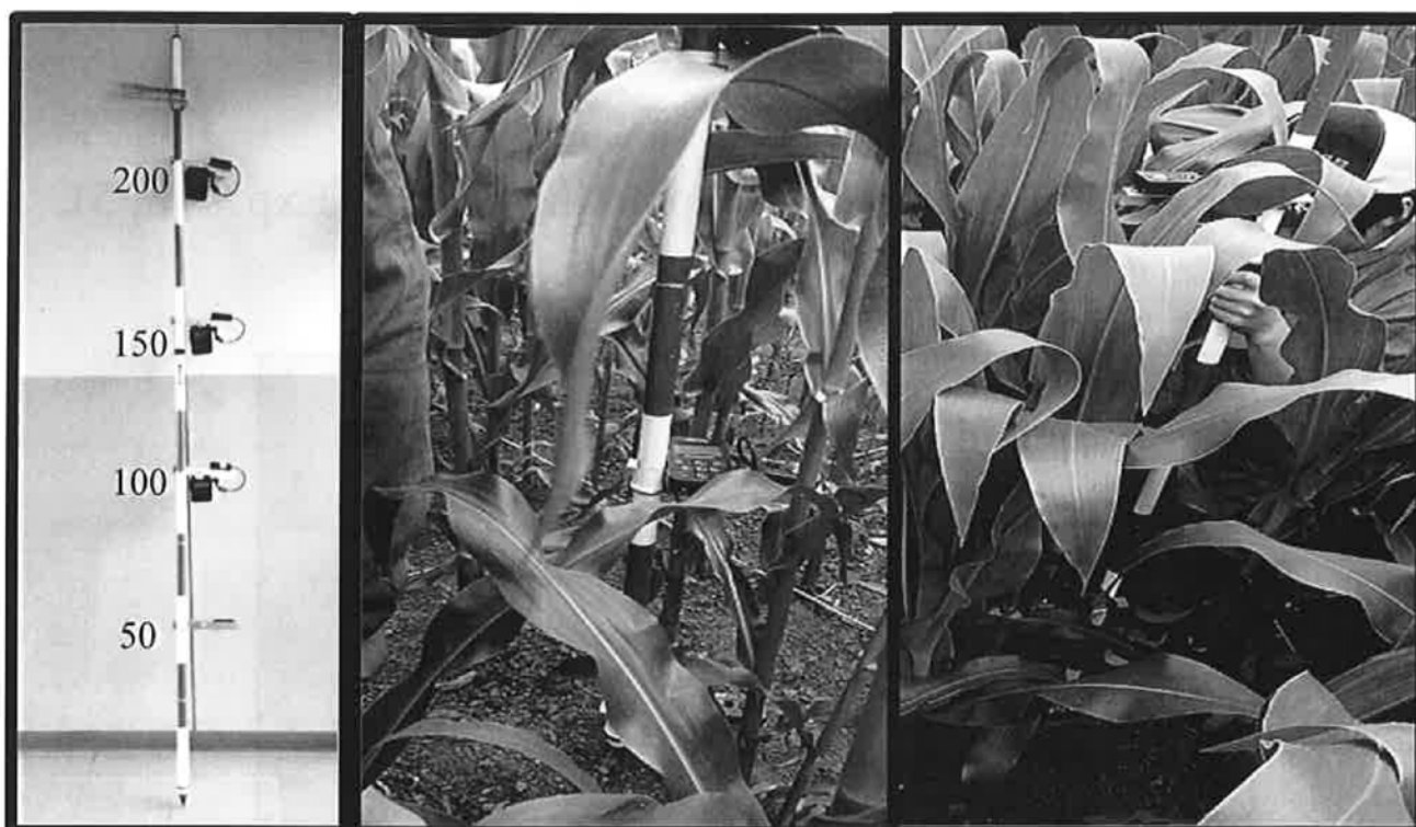
Fig. II -3 Measurement of relative illuminance in the plant canopy (Exp. 2).
