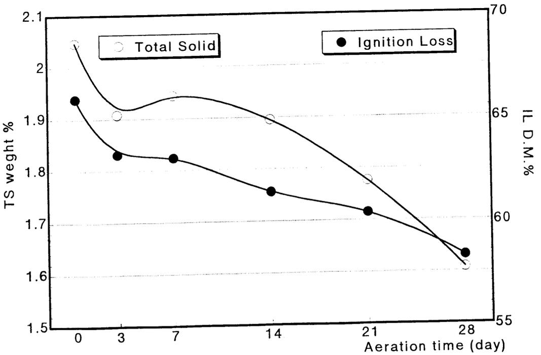
Fig. 8. Change in TS and IL of slurry during aerational treatment.
