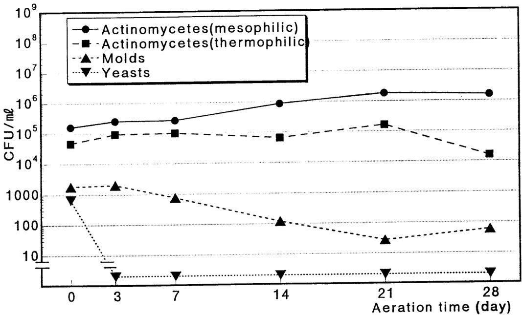
Fig. 5. Change in viable counts of actinomycetes and fungi during aerational treatment of slurry.
