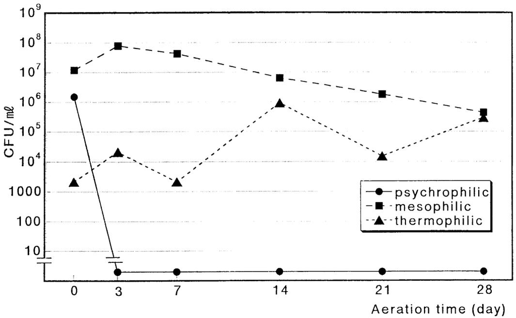
Fig. 2. Change in viable counts of aerobic bacteria during aeration treatment of slurry.
