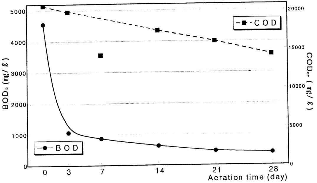
Fig. 7. Change in BOD<sub>5</sub> and COD<sub>cr</sub> of slurry during aerational treatment.
