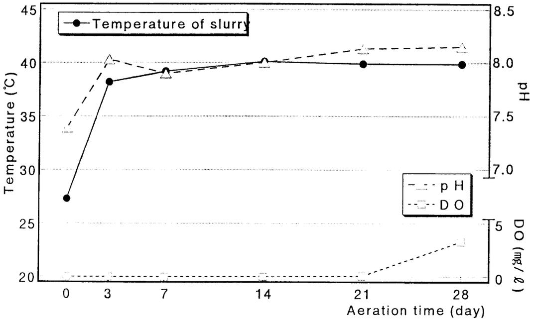
Fig. 6. Change in temperature, pH and DO of slurry during aeration treatment.
