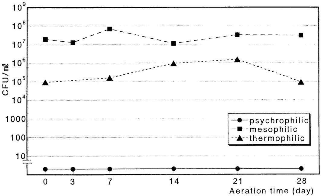
Fig. 3. Change in viable counts of anaerobic bacteria during aeration treatment of slurry.
