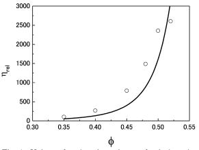
Fig. 4 Volume fraction dependence of relative viscosity for the model chocolate without emulsifier at a low shear rate (1.25 s<sup>-1</sup>). The line denotes the prediction based on the Krieger-Dougherty equation (Eq. 3)
