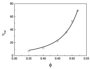
Fig. 3 Volume fraction dependence of relative viscosity of the model chocolate without emulsifier at a high shear rate (125 s<sup>-1</sup>). The line denotes the prediction based on the Krieger-Dougherty equation (Eq. 3)
