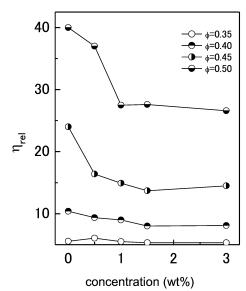
Fig. 9 The relative viscosity for the model chocolate with various volume fractions of silica particles containing ER-290.  $\phi$  denotes the volume fraction of silica particles in the system. The viscosities were measured at 125 s<sup>-1</sup> and 50 °C.
