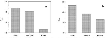
**Fig. 6** Effect of emulsifiers on relative viscosity at 0.125 s<sup>-1</sup> (a) and 125 s<sup>-1</sup> (b) for the model chocolate. The concentration of both lecithin and PGPR was 0.5 wt%.
