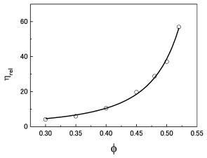
Fig. 7 Volume fraction dependence of relative viscosity for the model chocolate containing lecithin (0.5 wt%) at a high shear rate (125 s<sup>-1</sup>). The line denotes the prediction of the Krieger-Dougherty equation (Eq. 3).
