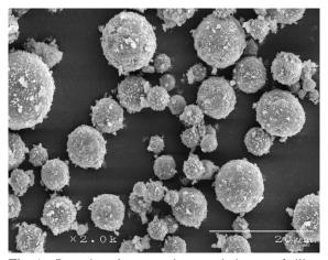
Fig. 1 Scanning electron microscopic image of silica particles used in the model chocolate.
