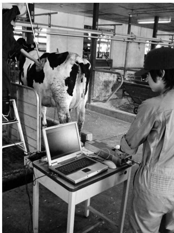
Figure 2-5 Techniques for measuring cone penetration resistance in rumen digesta.
