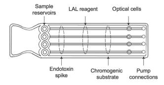
Fig. 2. The Endosafe<sup>®</sup> PTS System. The *limulus amebocyte lysate* (LAL) reagent cartridge for PTS. Kinetic chromogenic reagents and endotoxin controls are dried in the channels of a polystyrene cartridge. The specimen is pumped into the channels in which it is mixed with reagents and monitored for changes in optical density. Results are interpolated against an archived endotoxin standard curve.
