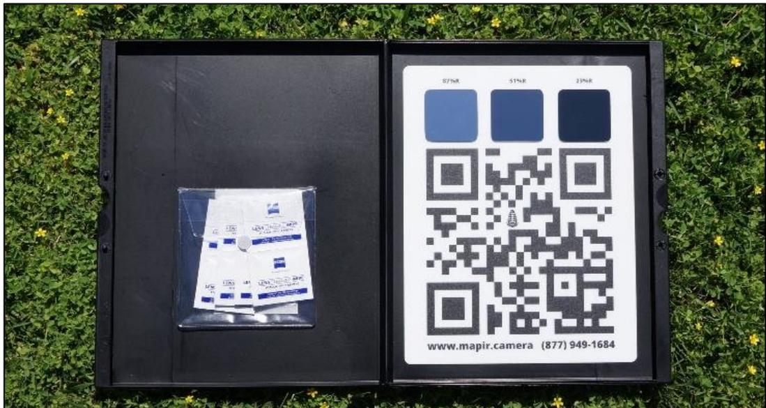
Figure 4: Mapir Camera Reflectance Calibration Ground Target
