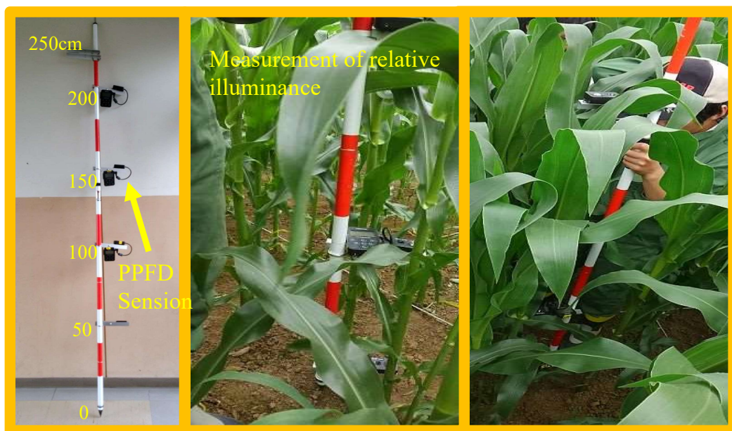
Figure II-4. Instruments used to measure the extinction coefficient, experimental scene in maize community and calculation method (Exp. 2, 6, 7).
