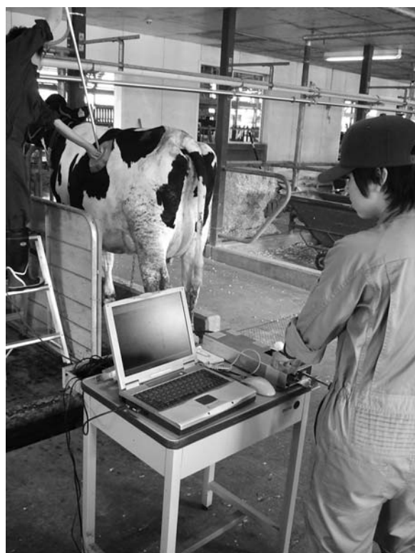
Figure 2 Techniques for measuring penetration resistance in rumen digesta.
